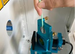
The 1st mirror is installed in the rear box of the laser tube, open it then view the right side.
