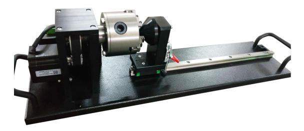
The chuck rotary axis attachment is the optional item.
