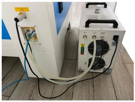
6 Add pure (distilled) water into the chiller until the water level in the green area showing on the gauge. Run chiller for a period of time, the water will fill into the laser tube on the machine, please re-add water to keep the water level in the green area.
