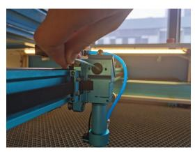
The 3<sup>rd</sup> mirror is installed on the top of the laser head.
