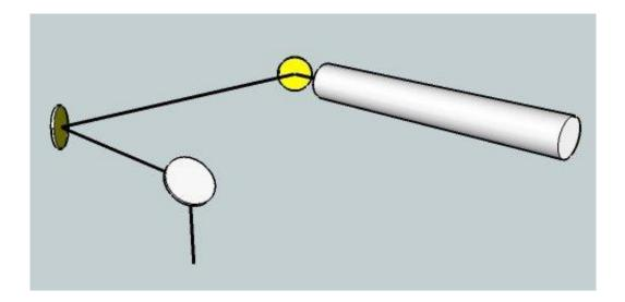
After being used for a long time, the beam path might be deflective. This will reduce the efficient of the laser beam or even cause no laser beam. At this moment, you will need to re-adjust the beam path again.
