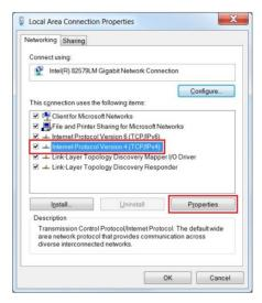
5). In "Internet Protocol Version 4 (TCP/IPv4) Properties" window, Select "Use the following IP address:"
