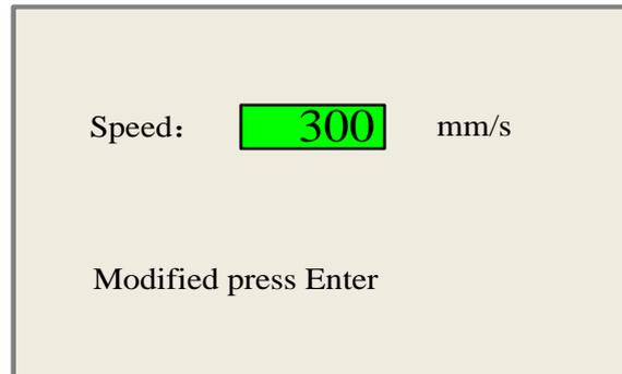
The speed is set from 0 to 1000mm/s, Push the "X+/-" Keys to move the cursor in the numeral area, and push the "Y+/-" keys to change the value, then push the "Enter" key to save the change, push the "Esc" key to invalidate the change.
