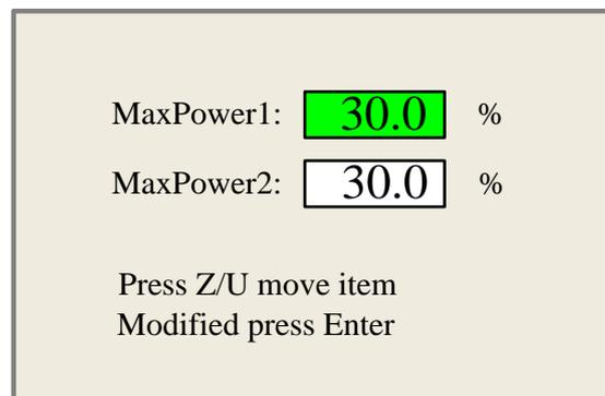
MaxPower1 is the power setting for the current laser tube; MaxPower2 is spare.
