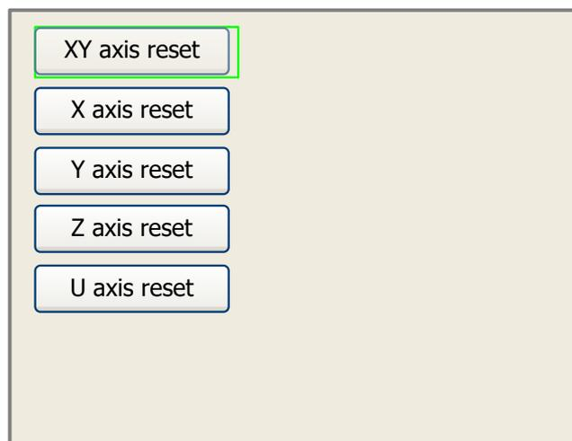
Press up and down arrow keys to move the cursor to one of the entry, then push “Enter” key to restart the selected axis, the screen will show some information when resetting.
