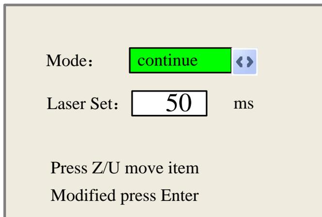
Push “Z/U” key to move the green block, and when the green block is on the “Mode” item, push “X+/-” keys to select the anticipated value, “Continue” or “Manual”. When “Continue” item is selected, then the “Laser Set” item is not valid, on that time, push the Laser key to splash the enabled lasers, and when Laser key is loosed, then the lasers will finish splashing. When the Mode item is “manual”, then pushing the Laser key one time, the enabled lasers will splash a fixed time.
